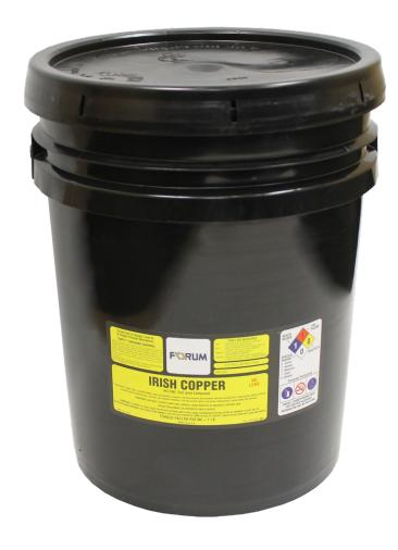
Forum Irish Copper no-lead tool joint compound is a copper-based, API RP 7A1 tool joint compound that employs a high-quality, low-sulphur petroleum base composition including anti-galling and anti-seizing agents. This compound is not affected by solvents, oil, mud, corrosion and mild acids or alkalies. Lead and zinc are not utilized in response to alternative "Lead Free and Zinc Free" compounds required by current industrial environmental safety standards.
