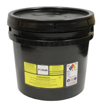
ForumSeal No-Lead/No-Zinc was developed as a special duty Teflon lubrication compound for casing threads. Lead and zinc were removed in order to provide a "Metal Free" thread compound mandated by current industrial environmental safety standards. ForumSeal No-Zinc meets or exceeds the performance requirements of API 5A4.
